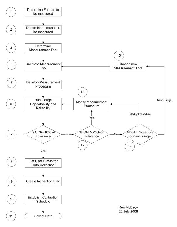
The feature chosen for inspection should have a tolerance called out on the print or specification. This tolerance will to a large degree determine the cost of the inspection equipment. If the tolerance is +/- 0.020 or a surface finish of 125 or a circularity of 0.020, the required accuracy and cost of the inspection equipment will be much less than if the tolerances are +/- 0.002 or a 8 surface finish or a
