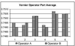
The first thing that I noticed from this data is the Micrometer had one reading that varied by 0.002. The total range variation for the Micrometer is 0.003. The readings from the Vernier look much closer on this sample. No penny varied more than 0.0005 between the four readings of the two operators. The total range variation for the Micrometer over all six pennies was 0.002.
