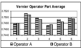
Reproducibility is a function of operator variation. In our sample, the electronic Vernier calipher shows less reproducibility than does the micrometer which means that the two operators were more consistent using the electronic Vernier than using the micrometer. The micrometer showed variation on parts 3, 5, and 6. The Verier showed variation on every part. The range of variation with either gauge was 0.004.
